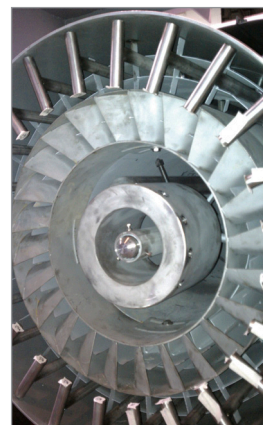
Internal view of a low-NO x burner for an industrial boiler.
